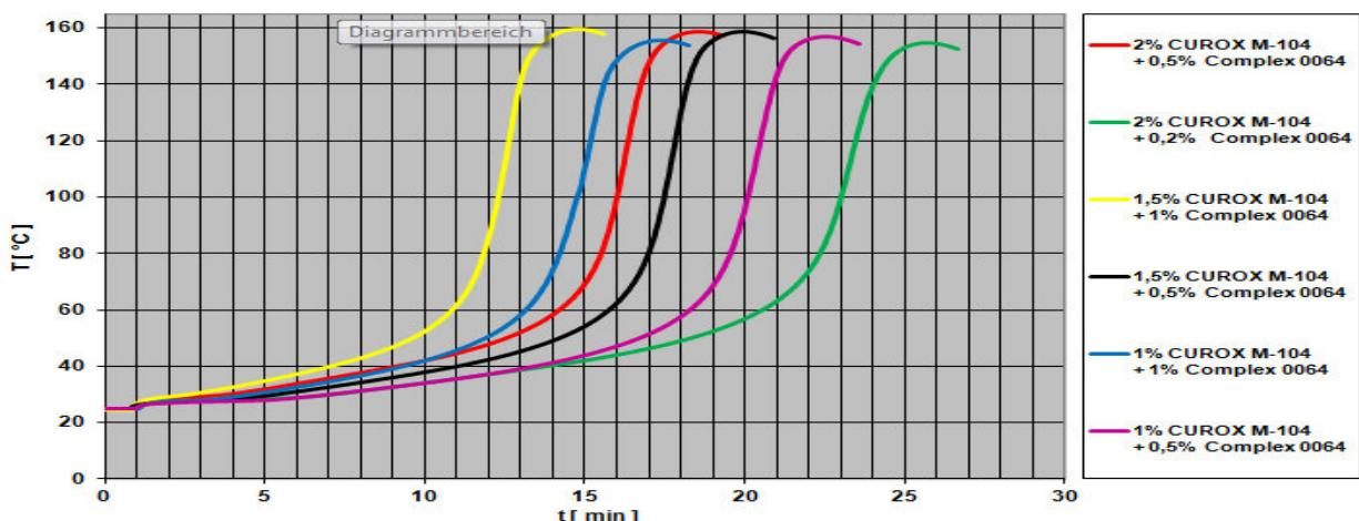
Measurements in compliance with DIN 16945 at 25°C with VE resin (20g in a test tube)
