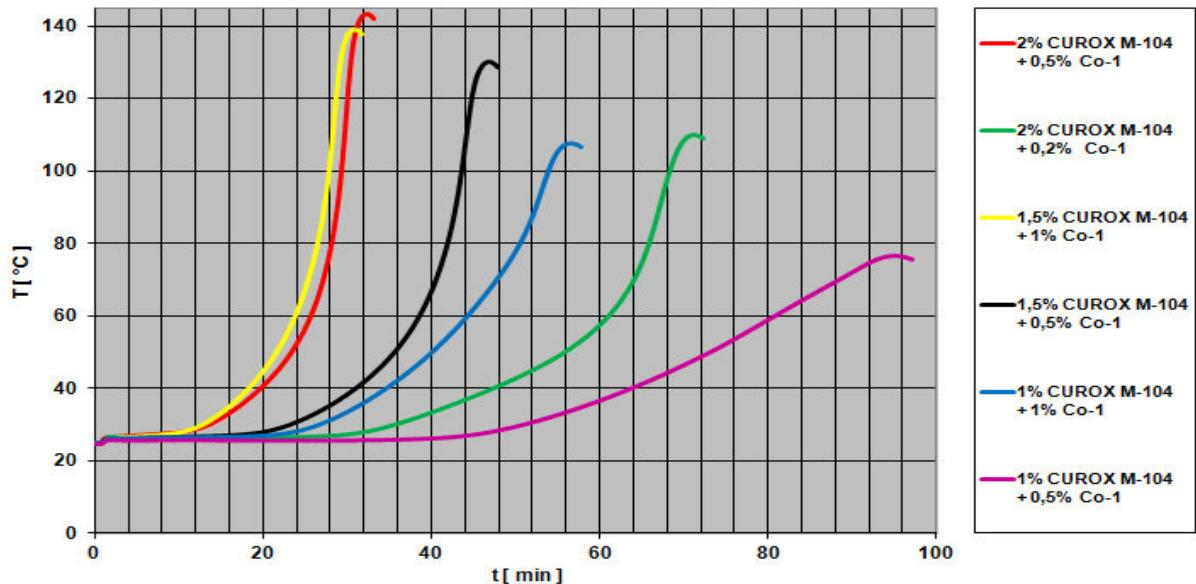
Measurements in compliance with DIN 16945 at 25°C with OPA resin (20g in a test tube)
