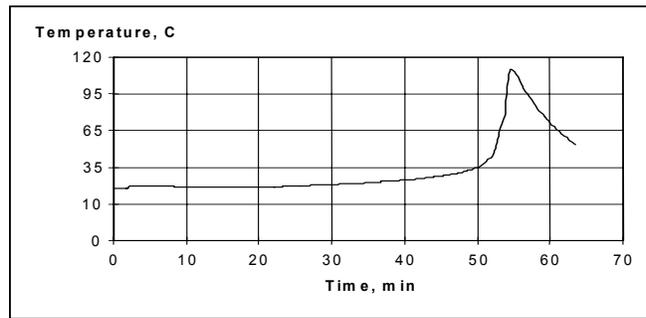
Typical Exotherm Curve for MA550 at 23°C (10 grams)<sup>5</sup>
